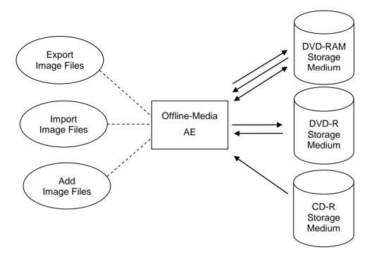
Figure 5.1-1 APPLICATION DATA FLOW DIAGRAM FOR MEDIA STORAGE
