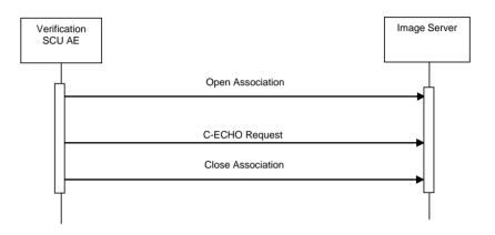
Figure 4.2-1 SEQUENCING OF ACTIVITY – VERIFY CONNECTIVITY
